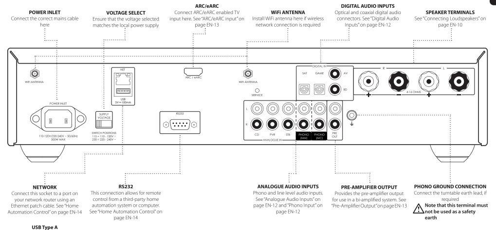
This USB socket is used playback of audio files from pen drives.
