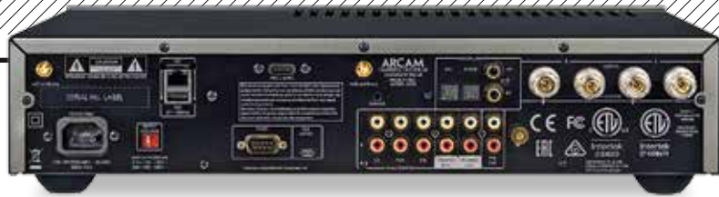
ABOVE: Comprehensive functionality is reflected in the three line/two phono inputs, two optical and two coax S/PDIF inputs, dual Wi-Fi antenna, wired network (for home automation/streaming) and USB-A (external HDD playback) ports, plus HDMI (ARC)
