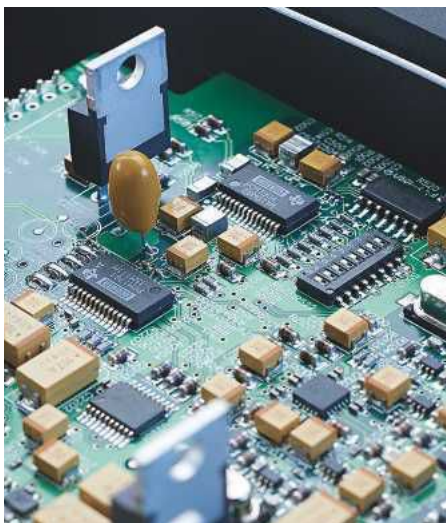
ABOVE: Analogue inputs are digitised via a TI PCM1804 ADC [top IC] while a companion PCM1791 DAC services the analogue outs
