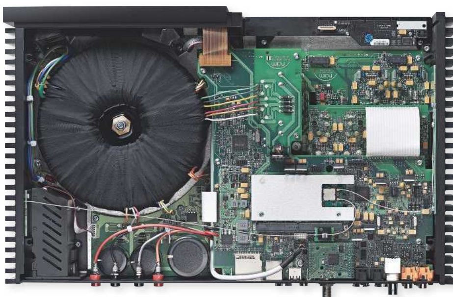
RIGHT: An over-sized mains transformer feeds linear PSUs for the analogue amplifier in addition to the SHARC DSP [centre], streaming board [silver, lower right] and ADC/DAC board [right]. A small switchmode PSU serves standby
